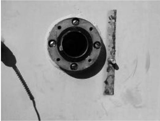
Into this well is inserted an inner well surrounded by a heating element powered by a bushing current transformer so that the heating corresponds to the KVA loading of the transformer.
