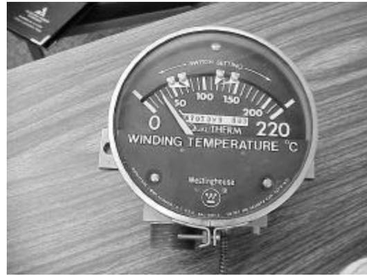
To make adjustments, a technician opens the glass and moves the pointer to where they want the action to occur. The contacts are generally configured as in the picture below
