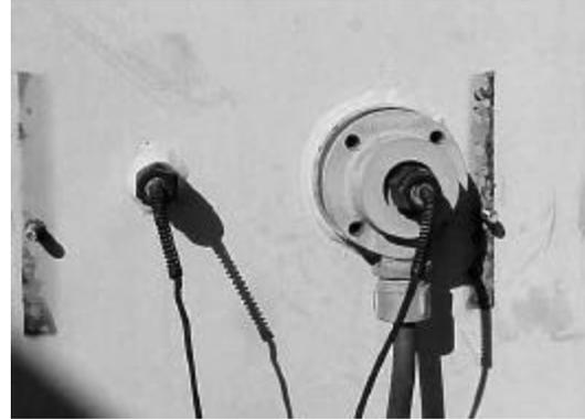
In the above picture, the top oil measurement probe can be seen to the left of the hottest spot probe inserted into the heated well.
