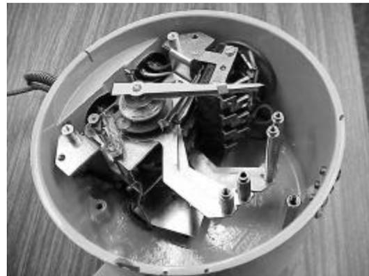
This system has functioned well for many years, but does have drawbacks in that setting the temperature correctly depends on the accuracy of the thermometer as well as the skill of the technician. Water and contaminants can enter the case over time and may corrode the parts and contacts causing failures. Newer replacement mechanical gauges may have plastic windows that cloud and become unreadable over time. Also, these instruments have no ability to provide an alarm if they become defective.
